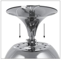
5. Hang the fan in the mounting bracket, ensuring that the ball joint locating groove aligns with the notch on the mounting bracket. Do not connect to supply.
